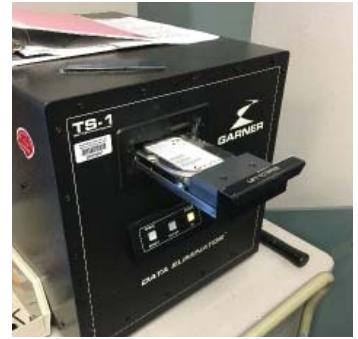
An agency degaussing hard drives before placing them in a secure shred bin.
